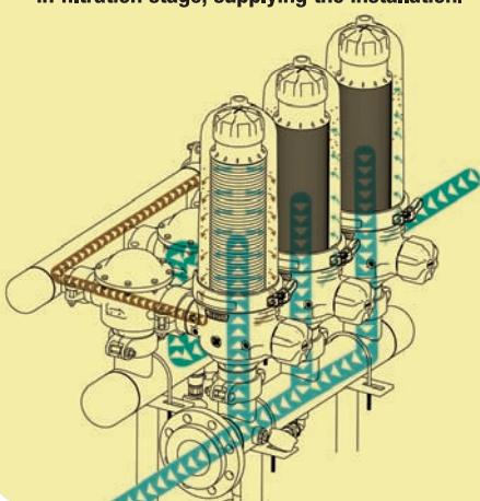
**FILTRATION STAGE:** The helix generates a centrifuge helical effect, which moves away from the discs the particles in the water.
